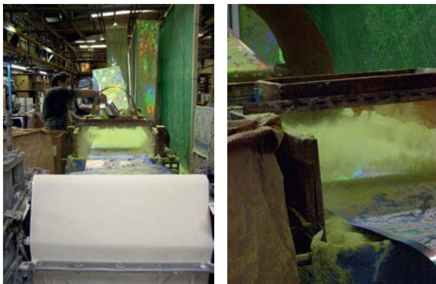
Figure 70. Flocking in process in the workshop of Cole & Son, Manufacturers of Handprinted Wallpapers from 1875.
