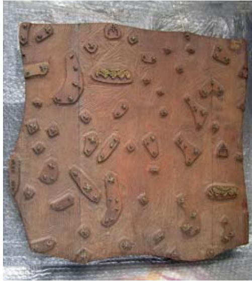
Figure 67. Fine details were printed with brass elements embedded in the block.
