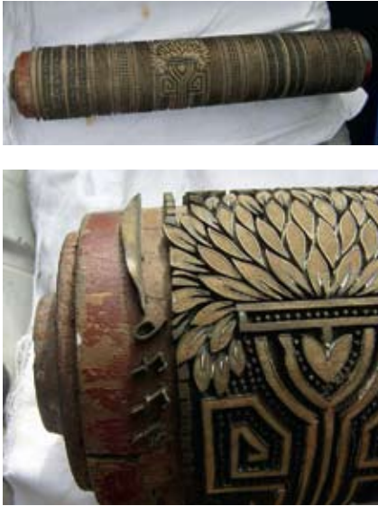
Figure 74. A surface-print roller for printing a fine Art Nouveau pattern. The outlines of larger areas are formed by stripes of brass. The number of pattern series is seen on the edge of the roller.
