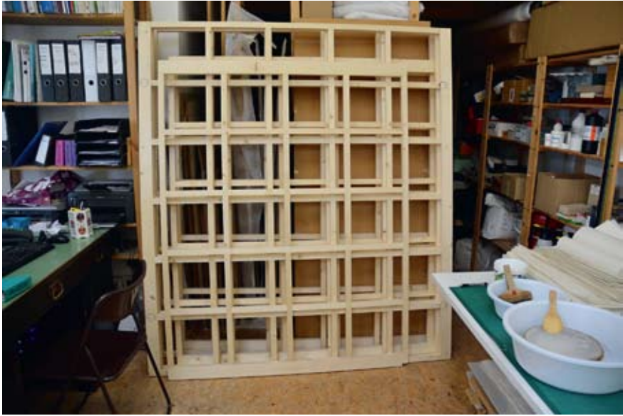
Figure 145. Japanese shoji frames before covering them with layers of Japanese tissue.
