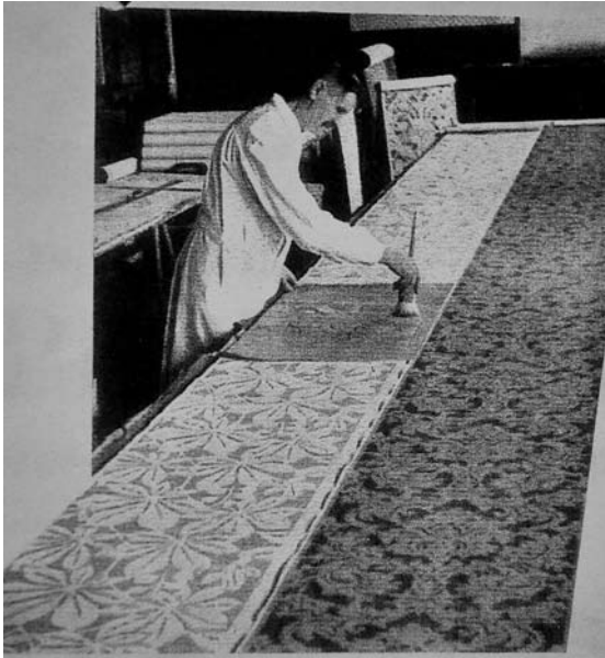
Figure 64. Stencilling is one of the most archaic methods of printings wallpapers. It is seldom used nowadays. Reproduction from Handbuch der Tapete , Franz Rullmann, Verlagsanstalt Alexander Koch GmbH, Stuttgart, 1958, p. 23.
