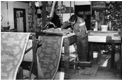
Figure 68. A block-printer producing a dado at John Perry's. Reproduction from The Wallpaper Review 1993/94, p. 24.
