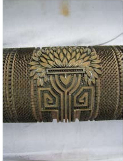
Figure 74. A surface-print roller for printing a fine Art Nouveau pattern. The outlines of larger areas are formed by stripes of brass. The number of pattern series is seen on the edge of the roller.
